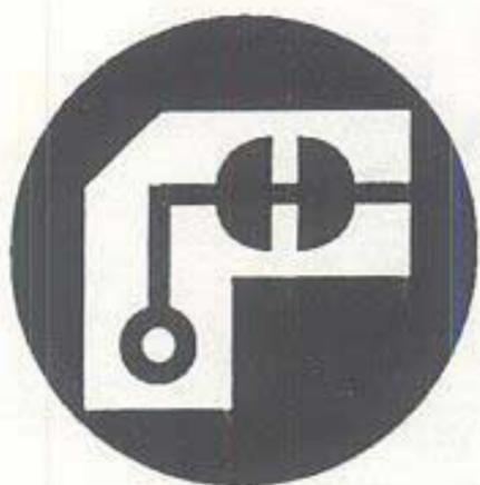
Cut the trace located between the two half-moons to use the higher capacity SIMMs.
